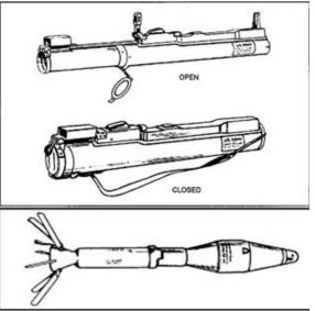
Outer Tube. The trigger housing assembly (which contains the trigger assembly) is on the upper surface of the outer tube. So are the trigger arming handle, front and rear sight assemblies, and the launcher's rear cover.
