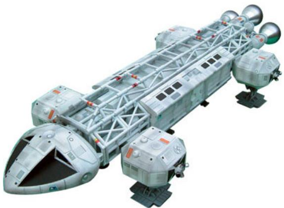
Description: Completely modular, the craft are divided into three basic sections: the command module, the service pod, and the superstructure (containing the landing gear, access corridor, aft compartment and main propulsion system).
